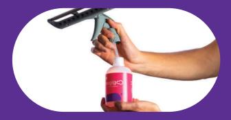
1. Remove the adhesive bottle and close with a cap.
